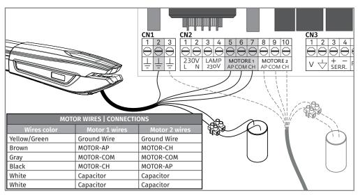
Connections should be made as shown above, connecting the 6 motor wires to the appropriate inputs of the control board and capacitor.
