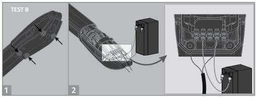
**Test B** • Loosen the 4 screws to remove the cover and access the internal connections. Make the connections as indicated in the image.
