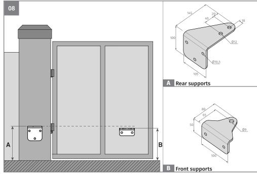
**Dimension A** • Vertical distance from the floor to the top of the rear support. **Dimension B** • Vertical distance from the floor to the top of the front support.
