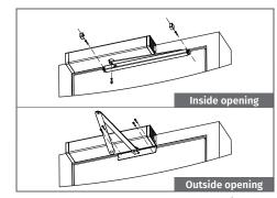
10 • Secure the arm on the automation and set the correct position of the guide to fix it in the door.
