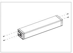
01 • Remove the 4 screws from the sides of the automation and remove the cover.
