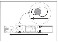
03 • Slide the automation to the left and separate it from the fixation plate.
