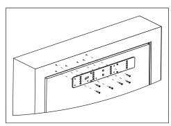
06 • Place the fixing plate directed with the holes and secure it with screws.
