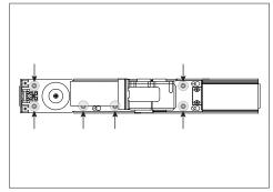
02 • Remove the 6 screws which hold the automation to the wall fixation plate.
