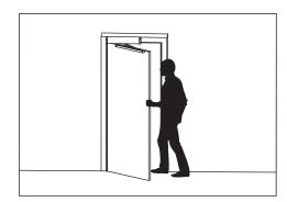
11 • Move the door manually to set the position of the opening stopper.
