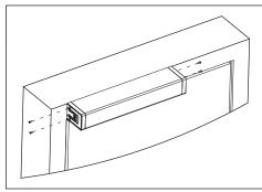
09 • Apply the cover on the automation and tighten the screws.
