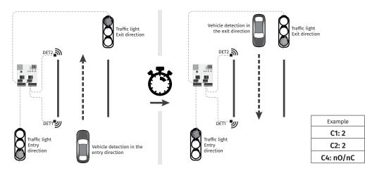
**Detection with PUL and DET inputs (detector operating mode only):** The detections on the track/road will be carried out by the DET and PUL inputs, in which the DET detects the entrance of the vehicle and the PUL detects the exit of the vehicle. This detection mode will allow you to have two different inputs and two outputs that at a given moment share a bidirectional road.
