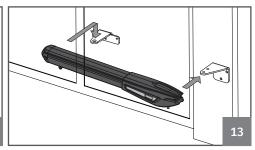
**02** • Install the automatism on the supports.
