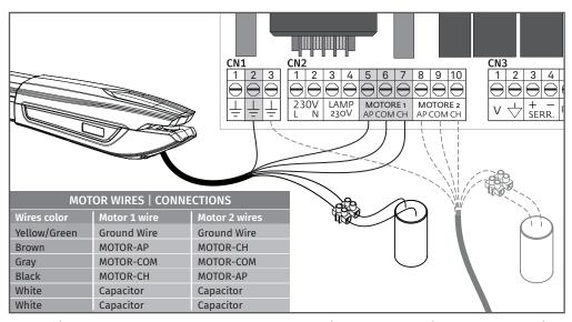
Connections should be made as shown above, connecting the 6 motor wires to the appropriate inputs of the control board and capacitor.
