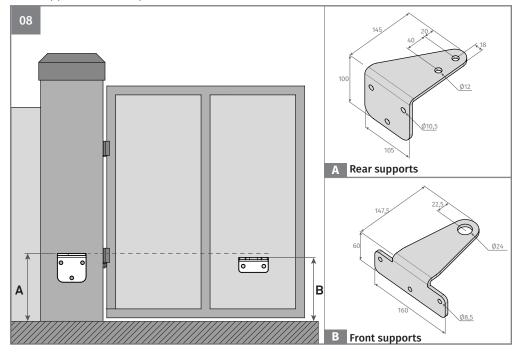
**Dimension A** • Vertical distance from the floor to the top of the rear support. **Dimension B** • Vertical distance from the floor to the top of the front support.
