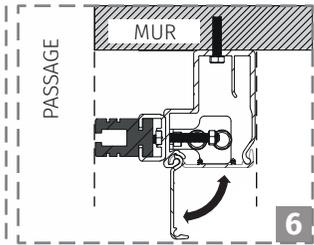
**6 FIXATION DES GUIDES AU MUR**
