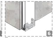
**G FIX LATERAL GUIDES TO THE GROUND** Start by drilling holes in the floor taking into account the holes already in the plates for the application of the screws. Finally, tighten the screws until the guides are
