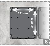
8 **FIX CONTROL BOARD** Determine the location for fixing the control board and fix it to the wall.
