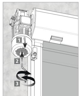
To open or close the door manually, simply pull and hold down the unlock lever and insert the crank, to turn the screw installed at the bottom of the motor (see image).
