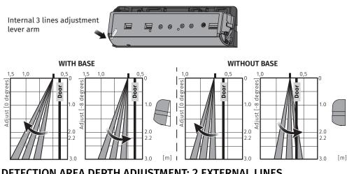
**DETECTION AREA DEPTH ADJUSTMENT: 2 EXTERNAL LINES**
