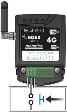
1 • Make a shunt between IN1 and IN2 and make a connection to as shown in the image;
