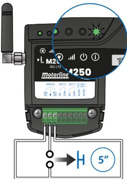
4 • You now have 5 seconds to open the circuit. The ACT Led will start to blink and you must keep the circuit open until the Led turns off again;
