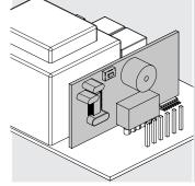
MR-12 with universal receiver - When triggered, the receiver always sends a NC start through a PULL contact.
