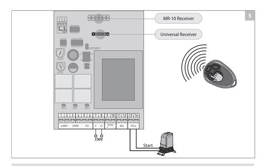
In case of having a universal receiver with external memory, it is possible to connect directly to a new Motorline control board, using the MR-12 interface as interconnection...
