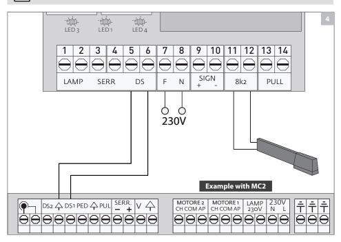
Some control boards (for example, MC2) are not prepared to receive 8K2 resistive type security bands. The use of MR-12 enables the connection of 8K2 resistive type safety bands and transforms it into NC contact.
