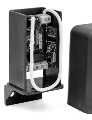
The MR17 receiver can operate electrical and electronic equipment remotely, with one or more commands (by radio).
