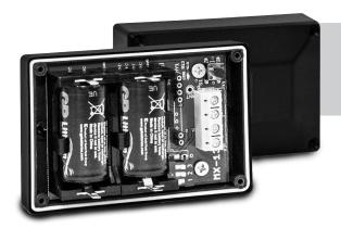
Wireless transmitter, which allows the connection of obstacle detection kits (safety rubber, magnetic contact, etc.), for communication with MR13. This device performs automatic operation tests with MR13, at defined time intervals, providing a longer battery life.
