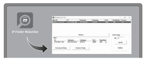
01 • Start the Motorline IP Tool software and search for the MRAC connected to your computer [Search button].
