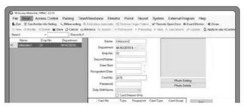
01 • In "Cardholder Info Setting" click [New] to create a new record and in the "Card No." field enter the desired PIN.
