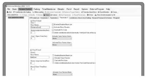
**08** • Activate the edit mode [Modify Button] and in "Parameter 3", activate the necessary doors and assign a name to each one. Save the changes [Save button].
