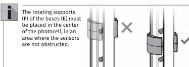
Place the photocell receiver (RX) in the place to be fixed, mark the 8 necessary holes in the supports of each photocell, drill and tighten.
